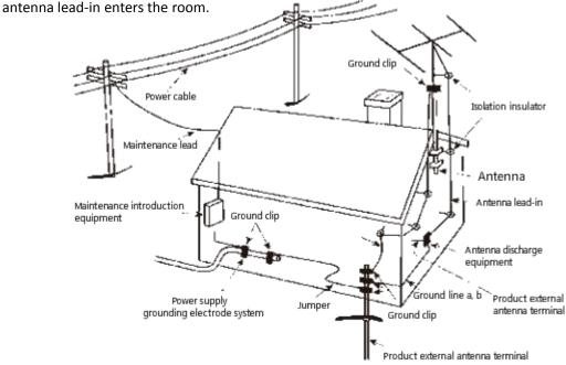
**Cable TV System Installation Instructions:** This instruction is used to alert the cable system installer to the National Electrical Code 820-40, which provides guidance on how to properly ground, especially when the ground wire is connected to the building grounding system. Near the wire lead-in point.
