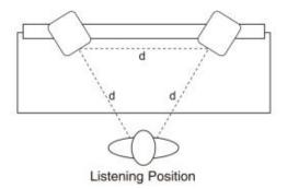
**Midfield configuration** - This configuration method is basically the same as the near field configuration. (See Figure 2.) The midfield configuration is usually used when the monitor speakers are large or when the monitor speakers are too large to fit on the mixer's bridge. This setting gives you a better overall position and better spatial audio and video effects. Make sure that the height of the woofer is higher than the height of the mixer's instrument bridge.
